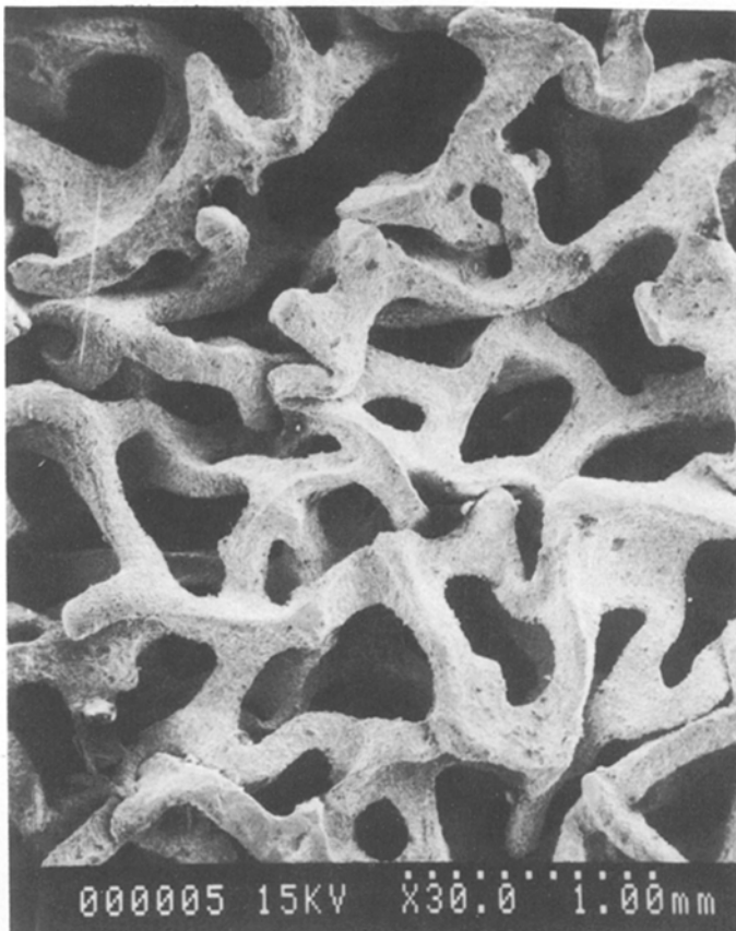
Figure 13 Scanning electron micrograph of re-entrant copper foam.
